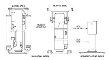
IMPORTANT: Do not use a dirty rag to wipe the jack rod or do not wipe the jack rod if it is coated with dirt. This could scratch and damage the rod. Make sure to use water or WD-40 to loosen any dirt before wiping the jack rod. If the jack rod has been greased or silicone sprays have been used on the jack rod, use WD-40 to loosen the grease or silicone and wipe the rod clean.
