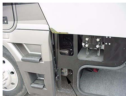
Hydraulic Pump Access - open storage compartment door behind driver's side front tire.
