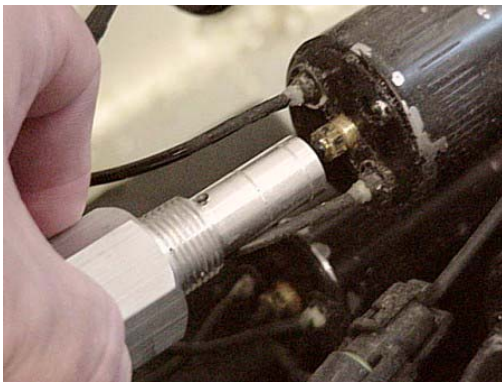
Use 1/4" nut driver built into end of pump reservoir cap to open slideout solenoid valves.
