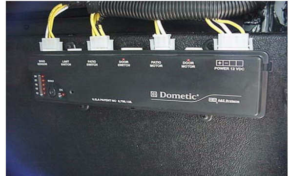
Awning Control Box (located in exterior compartment)
