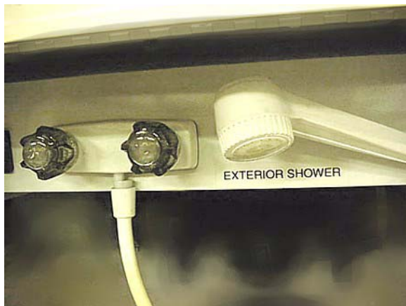
Exterior Shower/Wash Station (typical)
