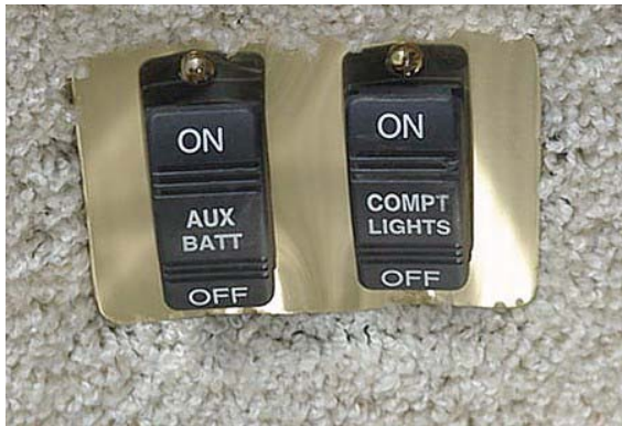
Compartment Lights Switch
