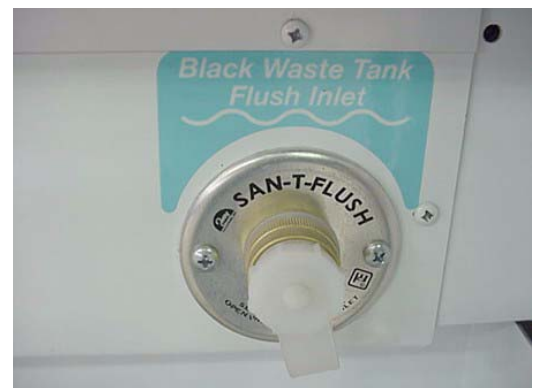
Water Tank Flush Inlet (typical)
