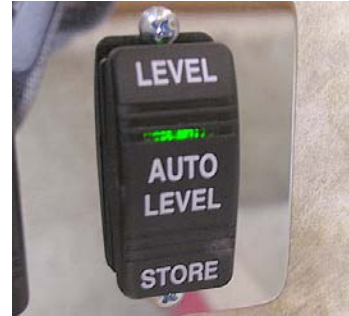
Auto Level Switch inside Entrance Door
