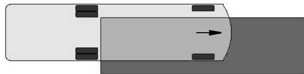
Weighing Right Front Corner
