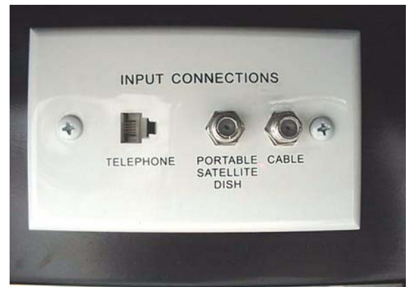
Exterior Connection for Phone, Satellite Dish and Cable TV (In Utility Compartment)
