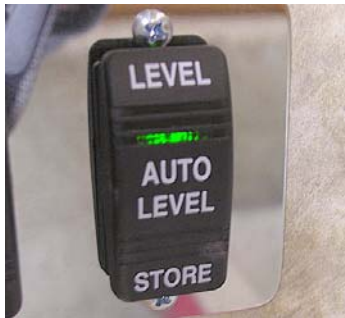
Auto Level Switch (Located inside entrance door)
