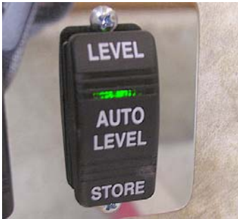
Auto Level Switch inside Entrance Door
