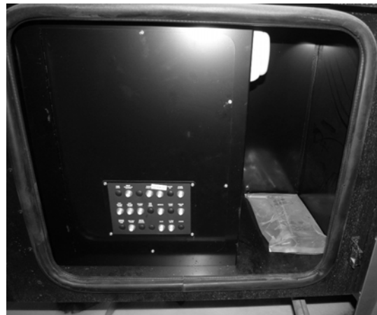
12-Volt Automotive Breaker Panel
