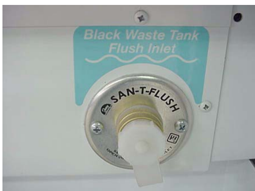
Water Tank Flush Inlet (typical)
