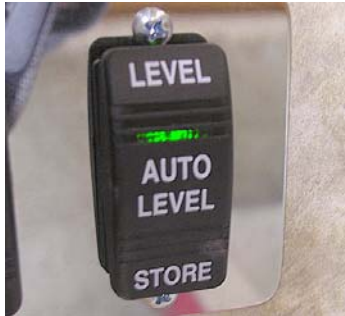
Auto Level Switch (Located inside entrance door)
