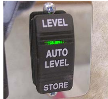
Auto Level Switch inside Entrance Door
