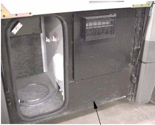
Water Pump Access Panel (typical)
