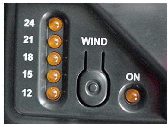
Wind Sensor Control Switch and Indicators on Control Box
