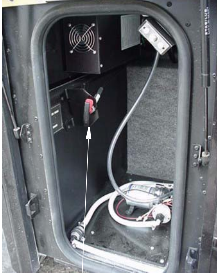
Water Tank Drain Valve- Model 38J (pull to drain)
