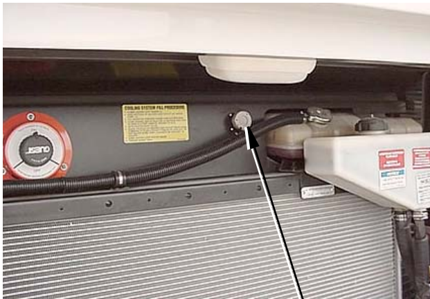
Diagnostic plug on rear engine compartment shroud
