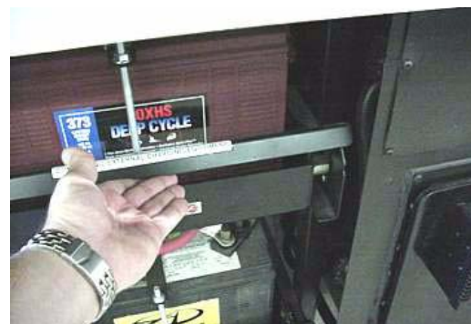
Lift Battery Tray Retainer Latches
