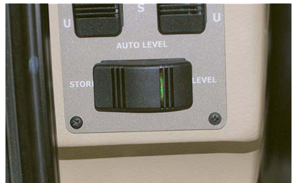
Auto Level Switch inside Entrance Door
