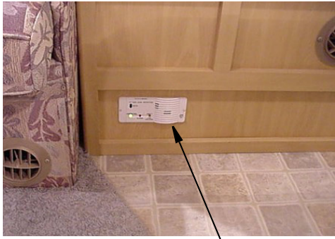
LP Gas Leak Detector
