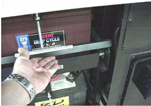
Lift Battery Tray Retainer Latches
