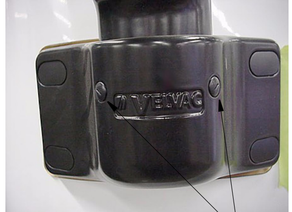
Remove (unscrew) caps to access set screws*
