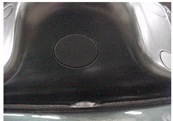
Carefully pry out plug on underside of mirror base to access pivot bolt.
