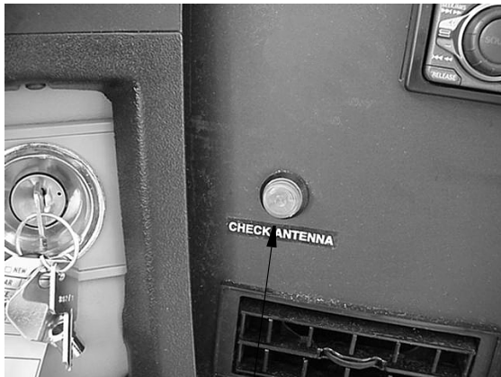
“Check Antenna” Light
