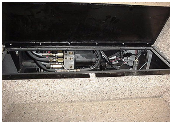
Hydraulic Pump beneath Entry Step
