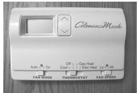
Gas Heat = Gas Furnace Electric Heat = Heat Pump Cool = Roof Air Conditioner
