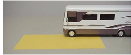
Weighing Left Front ‘Corner’
