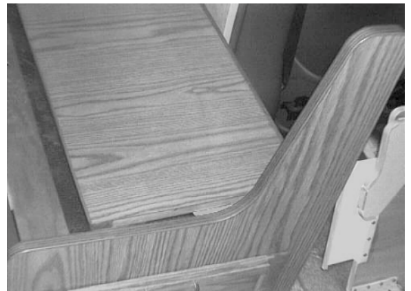
Dinette seat folds down to allow front seat reclining.
