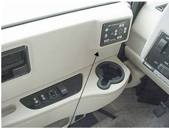
Hydraulic Leveling System Control Panel
