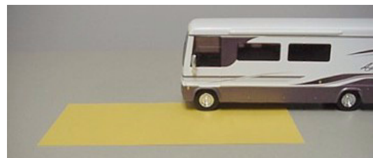
Weighing Left Front 'Corner'
