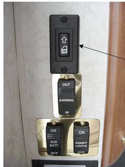
Power Lock Switch (near entry steps)
