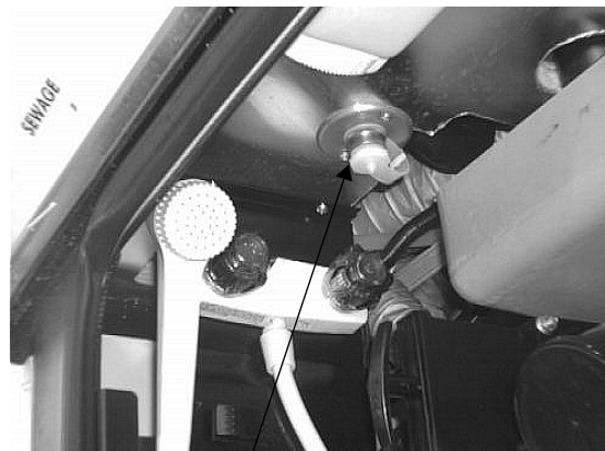
City Water Connection
