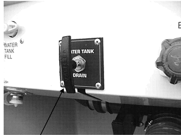
Water Tank Drain Valve (pull to open)
