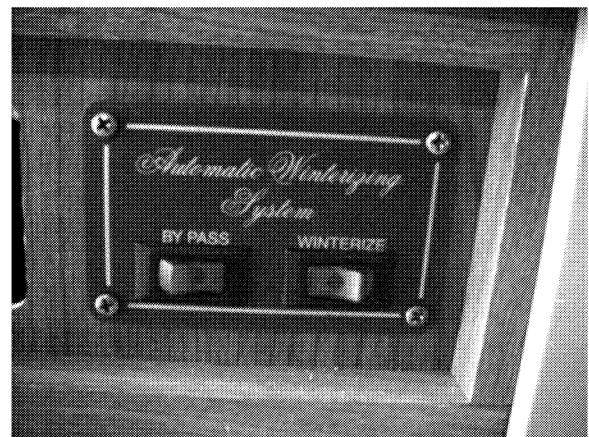
Winterization System Switches
