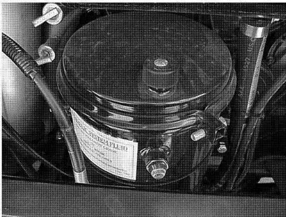
Hydraulic Fluid Tank
