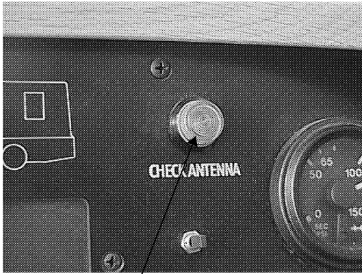
“Check Antenna” Light
