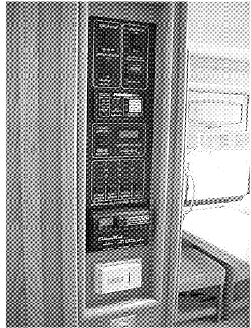
One Place Monitor Panel
