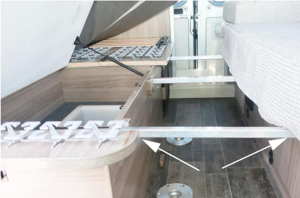
4. Place table top onto the support bars making sure the notch on the bottom of dining table aligns to the support bar.
