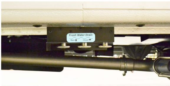
Waterlines and Tank Drain Valves
