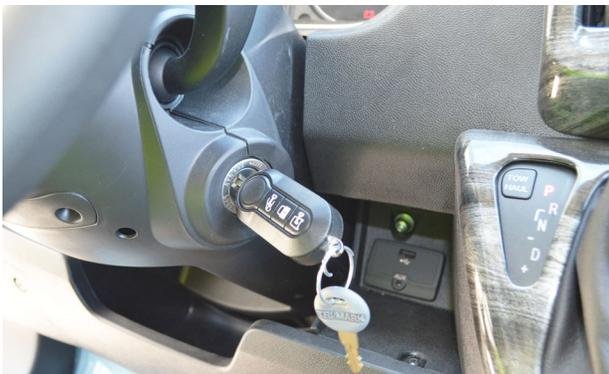
3. Leaving the key in crank position, push and hold the silver button on the left-side of the steering column for 2 seconds. Remove the key from the ignition. The horn will not sound.
