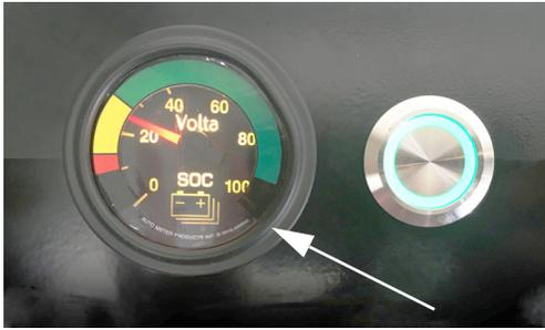
Pure<sup>3</sup> State of Charge (SOC) Gauge
