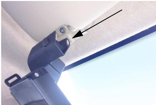
4. Lift the windshield pleated blind at the center handle to raise the shade into the fully extended position. If needed, adjust the rear view mirror to clear the shade.
