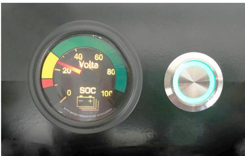
Pure<sup>3</sup> State of Charge (SOC) Gauge
