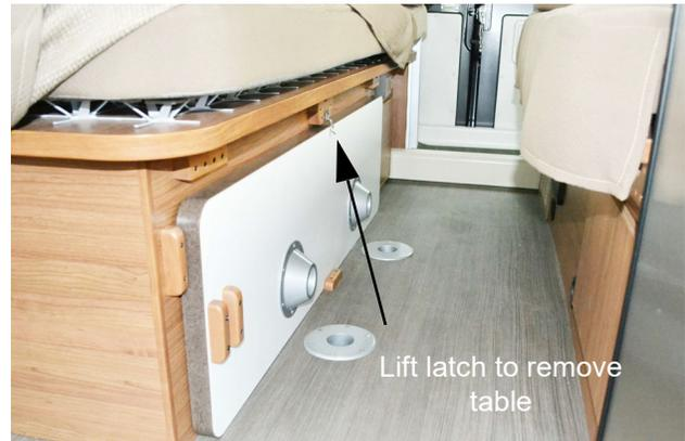
2. Remove the pedestal leg from beneath the passenger side twin bed cabinet.
