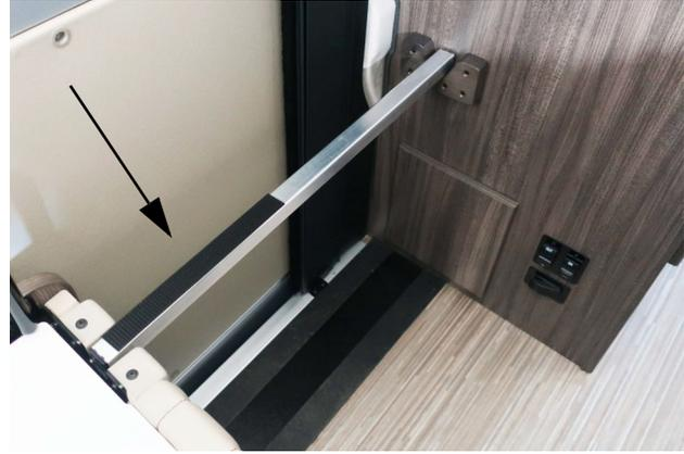
8. Align velcro on cushion and support bar. Push down to attach.
