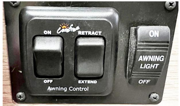
Power Awning control switches and Awning Light Switch
