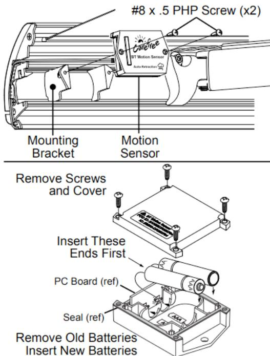
Awning motion sensor battery replacement
