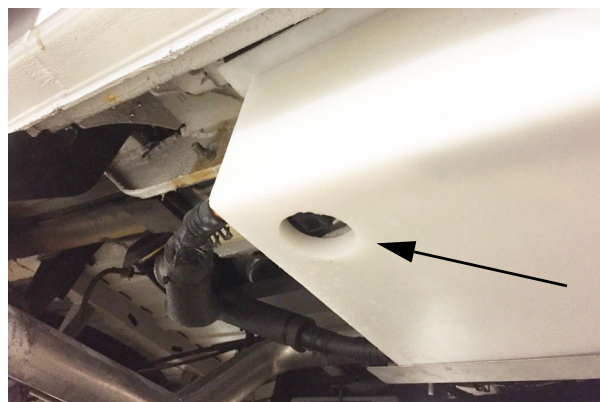
Water Tank Drain Plug (Located beneath running board, behind front passenger side door) -Typical installation shown
