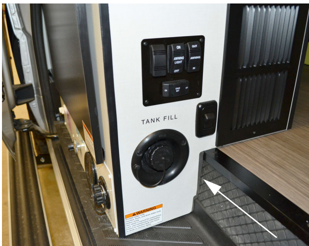
Water Tank Gravity Fill (Located near sliding entrance door)
