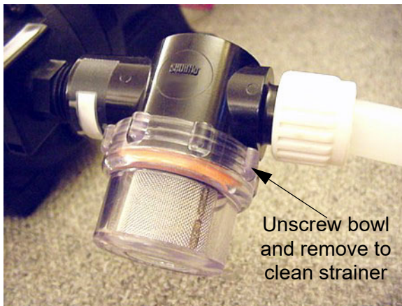
Water Pump Strainer -Typical View
