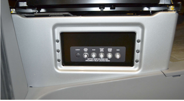
Automotive Chassis 12-Volt Circuit Breakers (Located on outboard side of passenger seat) * Shown with cover removed -Typical View
