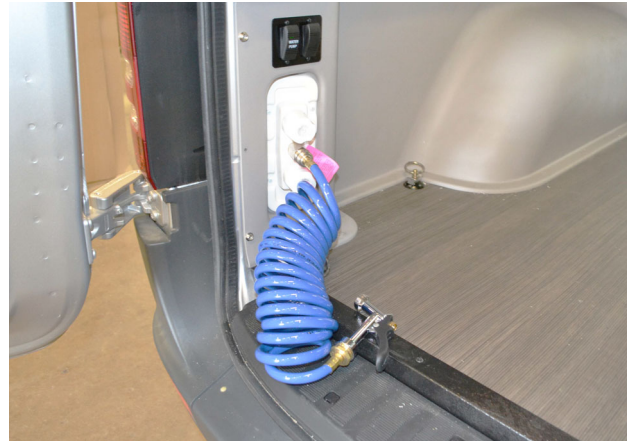
Exterior Shower/Wash Station Hot and Cold Water (Located inside the rear driver side door)
