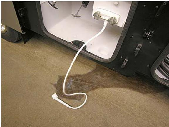
Using exterior shower to drain waterline
