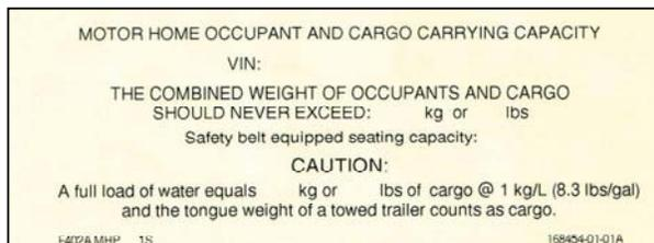
If any weight exceeding 45.4 kg (100 lbs.) is added to your coach between final vehicle certification and first retail sale, the occupant and cargo carrying capacity must be corrected and a label similar to the one shown below will be affixed inside your coach.
