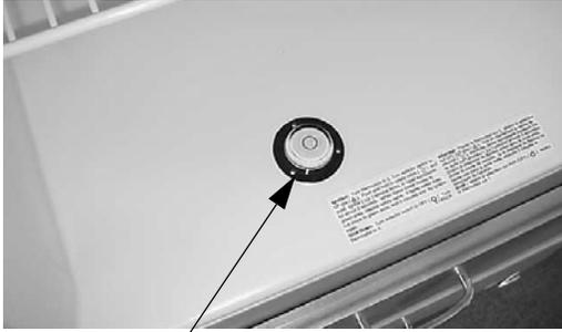
Place bubble level in bottom of refrigerator
