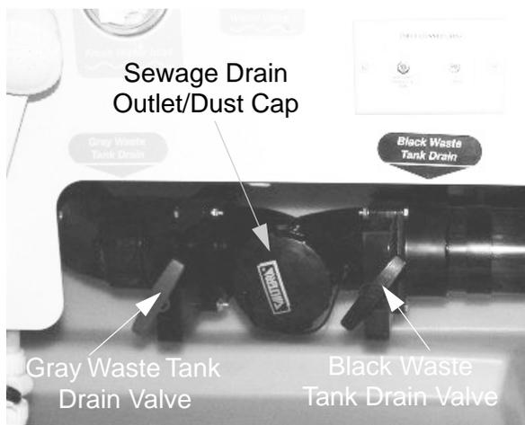
**Holding Tank Drain Valves
