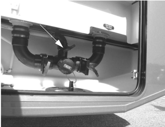
Black Waste Tank Drain Valve #2 (Front)
