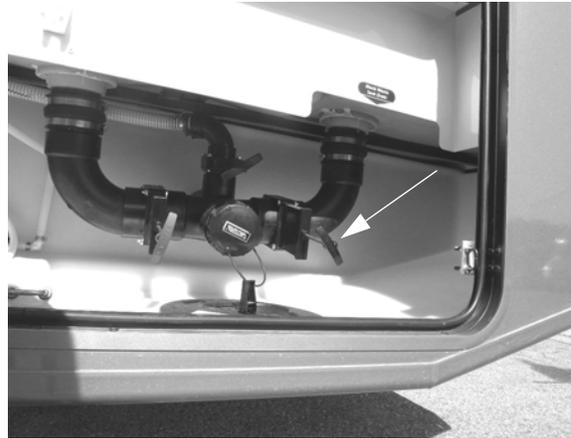
Black Waste Tank Drain Valve (Rear)
