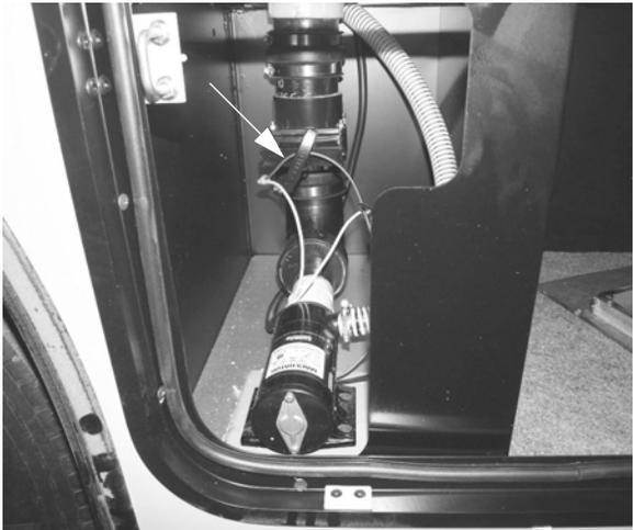
**Black Waste Tank Drain Valve #1 (Front)**
