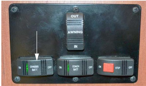
Chassis Battery Disconnect Switch
