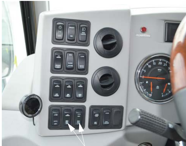
Engine Brake Activation Switches (Located on driver side trim panel) -Typical View
