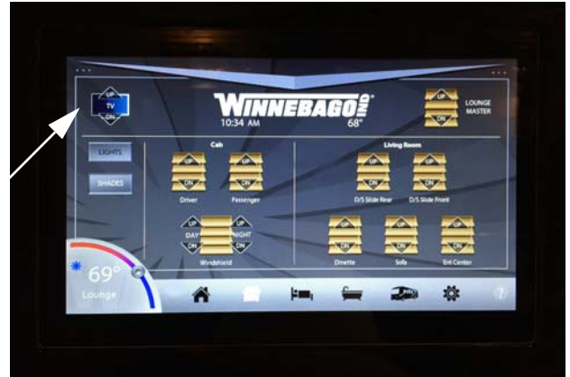
Buffet TV Power Lift/Lower Control Switch (Located on touch tablet "Lounge" screen)
