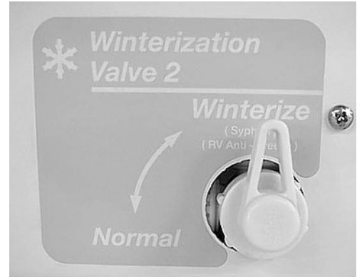
Winterization Valve 2 (Located near water pump - second compartment on driver side of coach)
