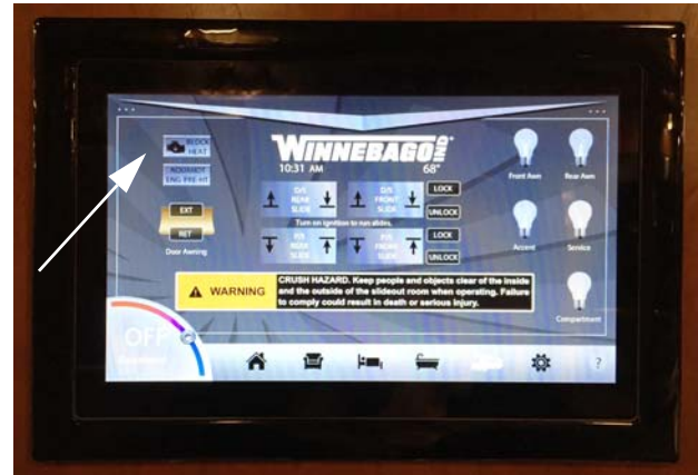
Diesel Engine Heater Switch (Located on touch tablet "Exterior" screen)
