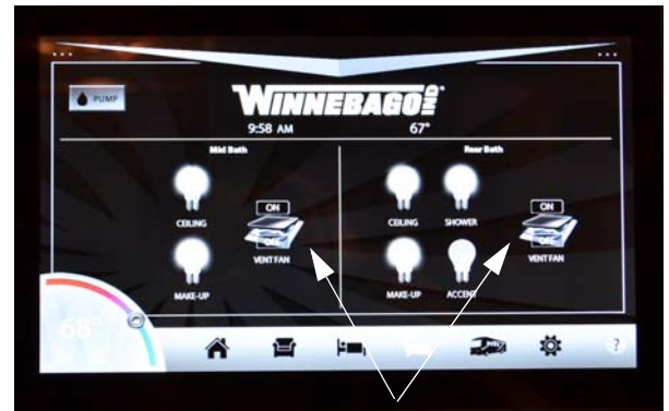
Power Roof Ventilator Switch (Located on touch tablet “Bath” screen) -If Equipped
