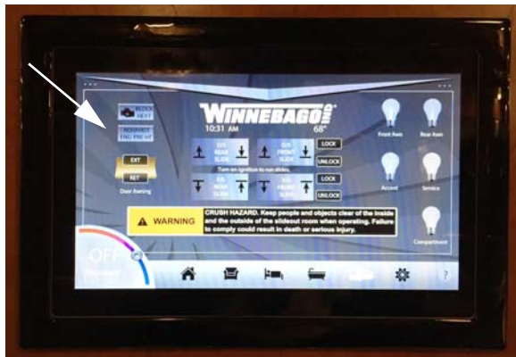
Hydronic Heating System Interior Control Switches
