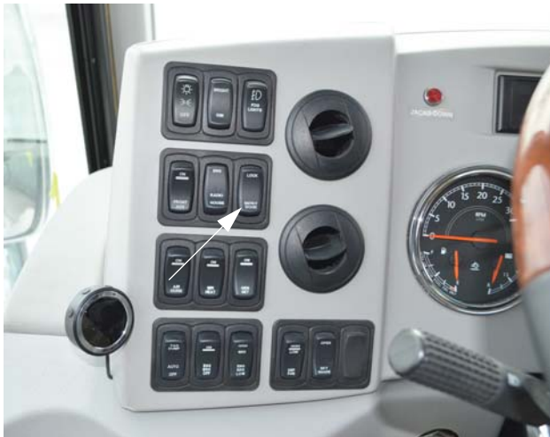
Power Door Locks - Entry Door (Located on dash) -Typical View
