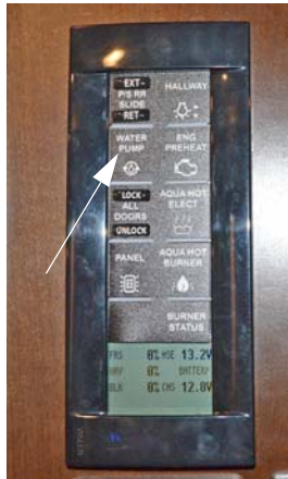
Water Pump Switch (Located on exterior water service center) -If Equipped The switch will illuminate blue when the switch is on. White illumination indicates the switch is off.
