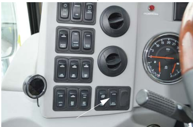
Skylight Shade Control Switch (Located on dash)
