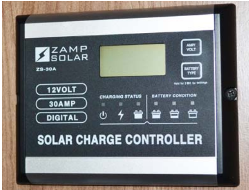
Solar Charge Controller (Located near monitor panel or in an exterior compartment, depending on model)
