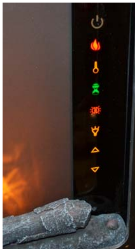
Fireplace Control Panel (Located on right side of fireplace)
