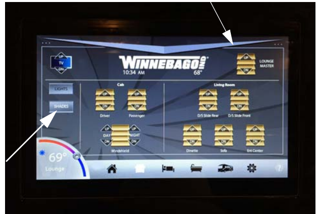
12-Volt Night Shade Switches (Located on touch tablet)
