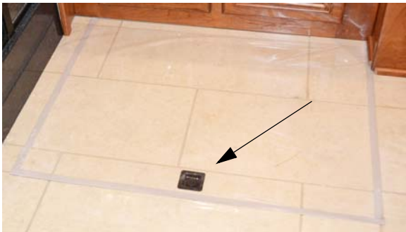
Engine Cover Latch -Typical View
