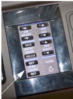
Step Cover Switch (Located on driver side trim panel) -Typical View
