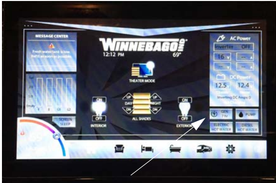
Generator Switch (Located on “Home” Screen)
