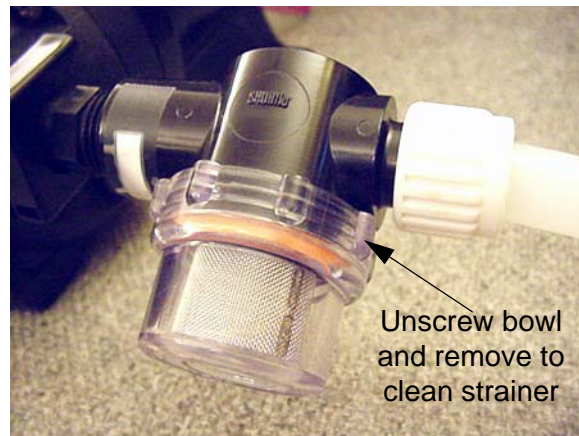
Water Pump Strainer -Typical View
