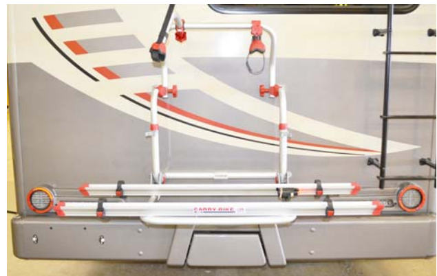
Pull straight down to lower bike rack for use. (shown in down position)
