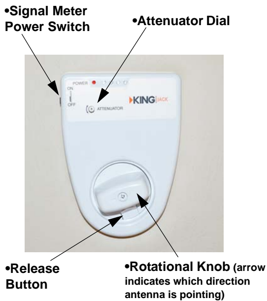
Digital Antenna Signal Meter (Located on ceiling)
