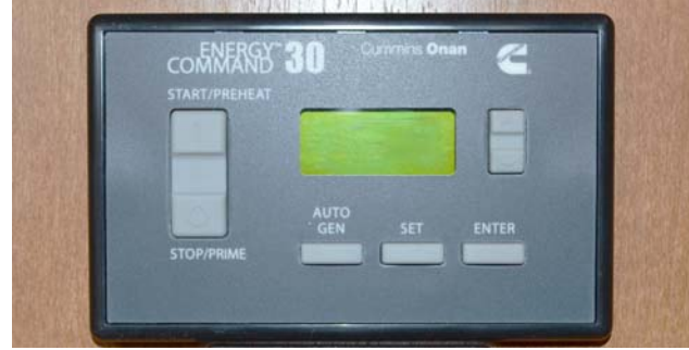
AGS Control Pad (Located near monitor panel)
