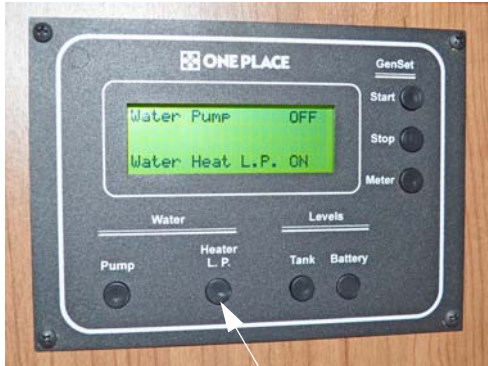
LP Gas Water Heater Switch
