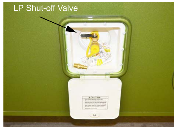
LP Accessory Connection • Model 27B and 31C - Located behind LP Tank access door on passenger side of coach.
