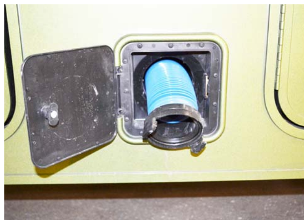
Sewage Drain Hose
