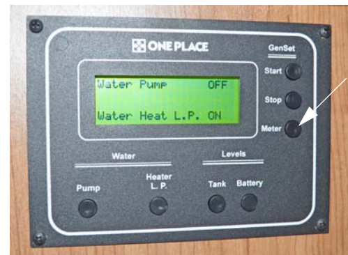
Generator Hourmeter Button -Typical View
