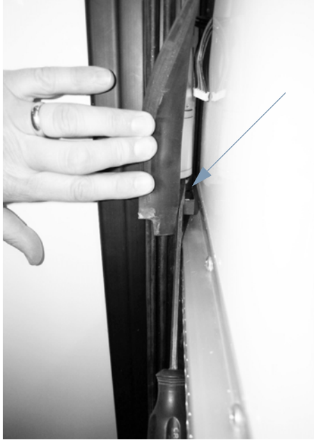
Slideout Motor (Located behind slideout wipe seal)
