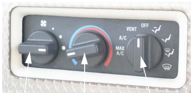
Blower Control Temp Control Mode Selector
