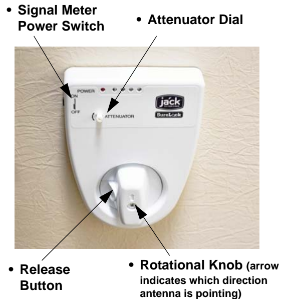
Digital Antenna Signal Meter (Located on ceiling)
