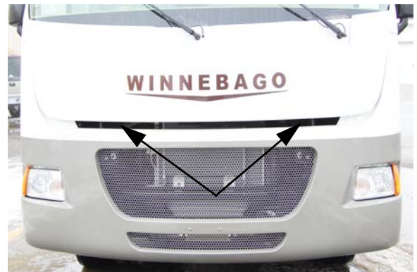
(Lift up the latches on each side of interior hood and raise) -Typical View
