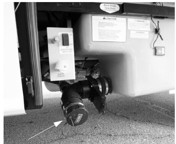
Sewage Drain Outlet/Dust Cap (Located in driver side compartment) -Typical View
