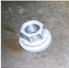
Six Chassis Supplied Lug Nuts with attached washers (located in the co-driver foot well compartment)
