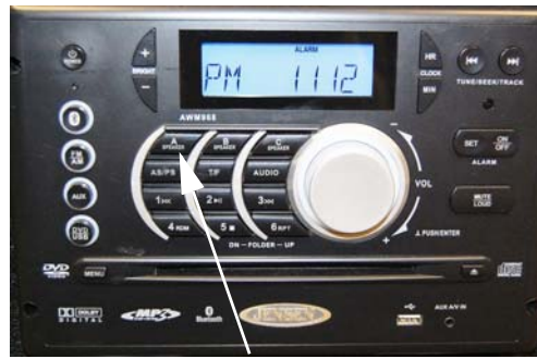
Interior Speaker Switch “SPEAKER A”
