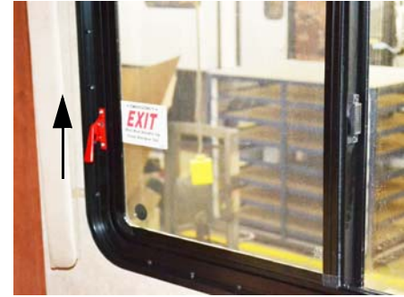
Escape Window Pull Red Handle Up and Push Window Out. -Typical View
