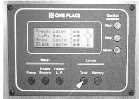
Tank Levels Switch
