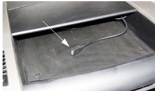
USB Cable (Located in compartment above dash radio) -Typical Installation
