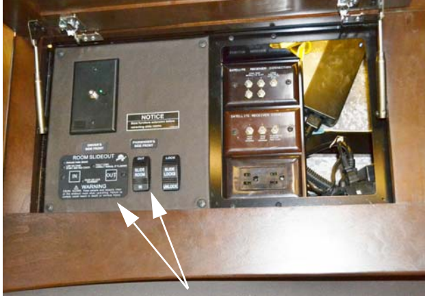
Front Slideout Switches (Your coach may have one or more of these switches depending on model, options, and available equipment) -Typical View
