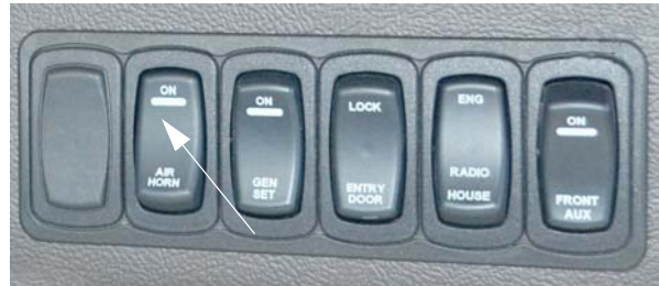
Air Horn Switch (Located on dash or driver side trim panel) -Typical View
