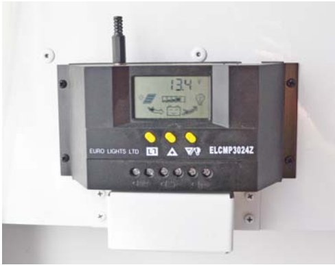
Solar Charge Controller (Located in utility compartment)
