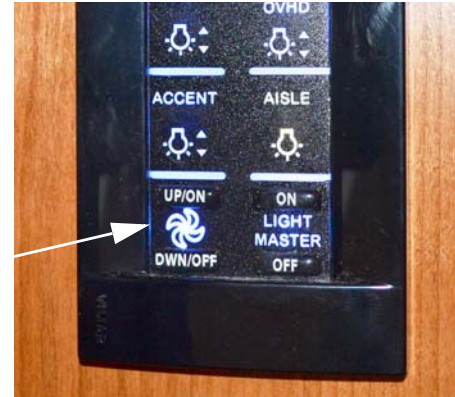
Power Roof Ventilator Switch
