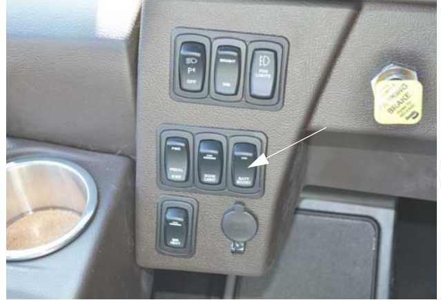
Battery Boost Switch (Located on dash)
