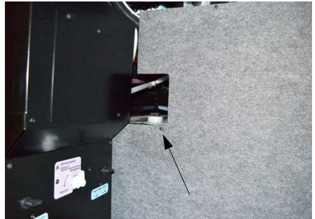
Gravity Fill Port (Located in the third passenger side compartment)
