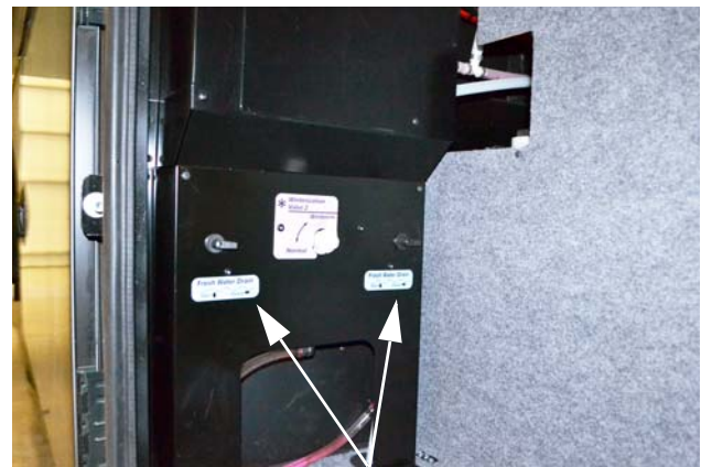
Waterline Drain Valves (Located in the third passenger side compartment) -Typical View
