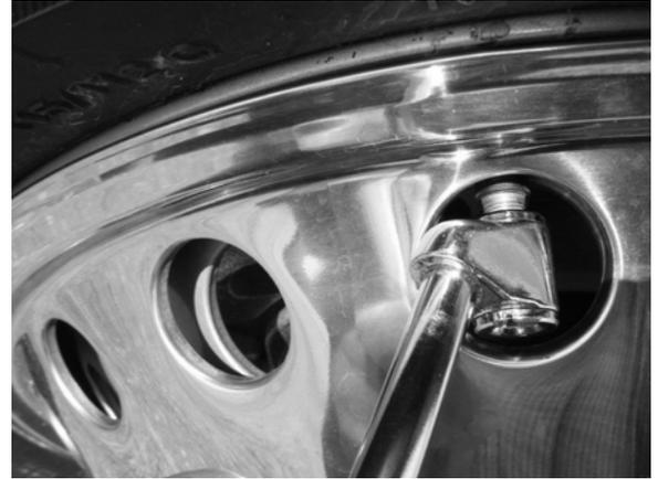
6. When tire pressure testing is complete, reinstall the valve stem cap (with the cap still retained in the hose extension end).
