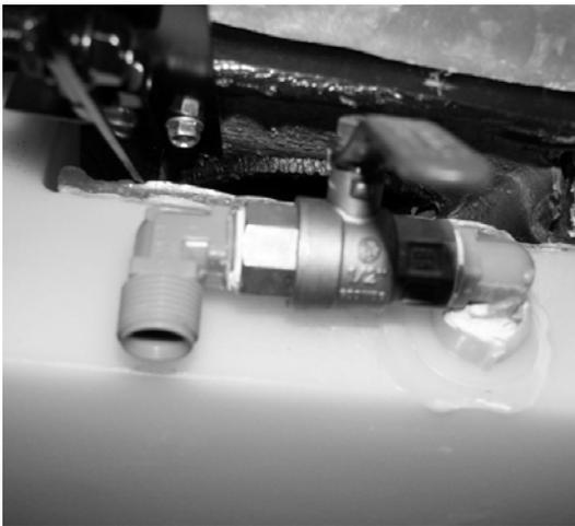
Water Tank Drain Valve
