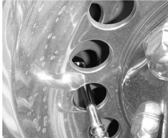
6. When tire pressure testing is complete, reinstall the valve stem cap (with the cap still retained in the hose extension end).
