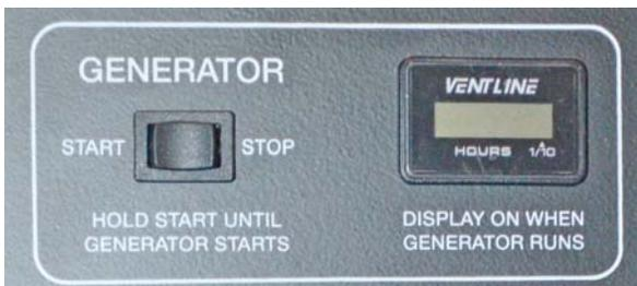
Generator Switch and Hourmeter
