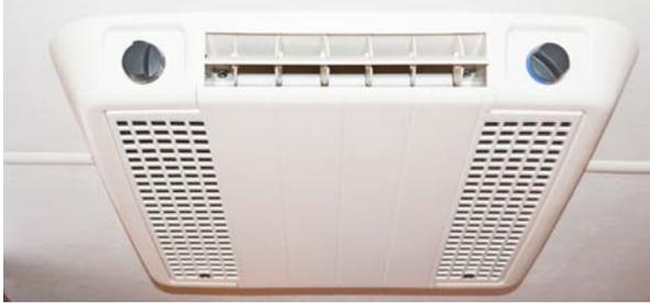
Your coach may be equipped with an air source heat strip built into the air conditioning system. Because the heat strip operates on electricity, it provides economical heat inside your coach and helps reduce the use of propane gas for heating in cooler weather.
