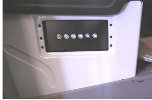
Automotive Chassis 12-Volt Circuit Breakers
