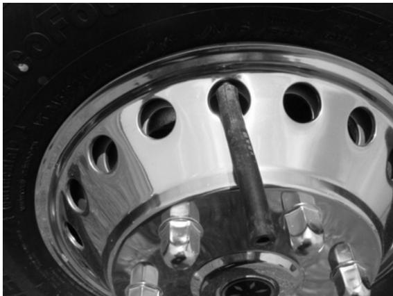
4. Using the hose extension as a remote handle, unscrew the valve stem cap (retaining cap in the end of the hose extension).
