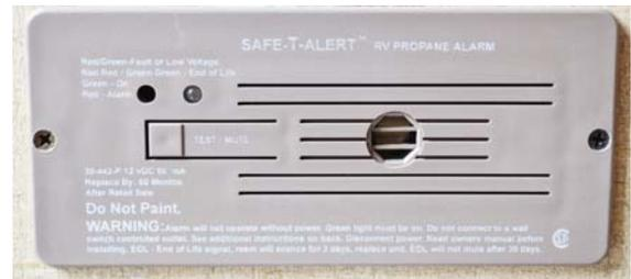
Propane Gas Leak Detector
