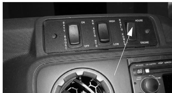
Radio Power Switch (Located in dash area) -Typical View
