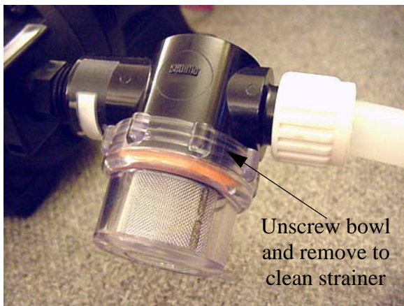
Water Pump Strainer -Typical View
