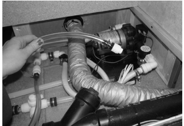
RV Antifreeze Siphon Tube (Located near water pump) * Insert into container of RV water system antifreeze
