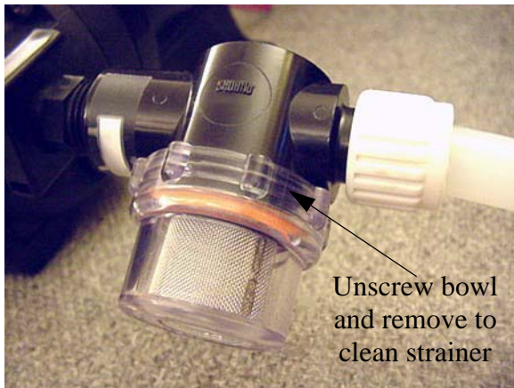
Water Pump Strainer -Typical View
