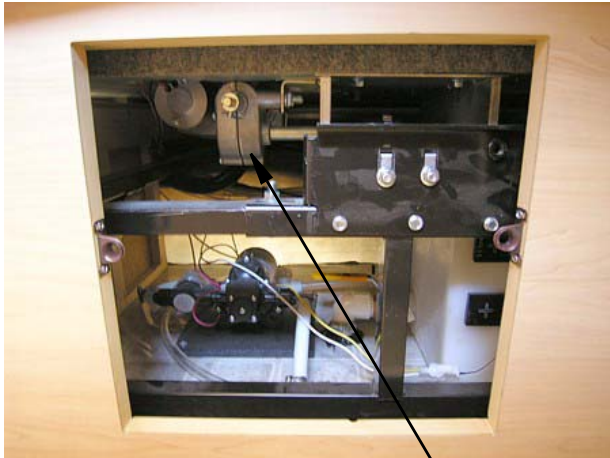
Rear Slideout Motor/Gear Location (behind pull-off panel at foot of bed base)
