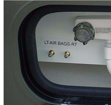
Rear Air Helper Spring Valves (Located in water service center compartment) -Typical View
