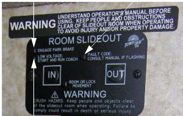
Low Voltage Indicator
