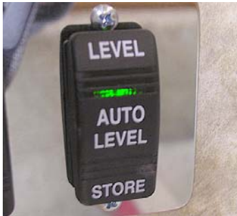
Auto Level Switch (Located inside entrance door)
