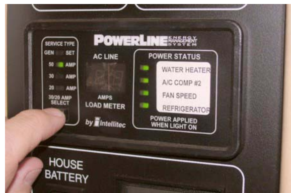
PowerLine EMS Display on Monitor Panel - Typical
