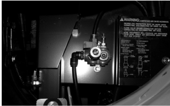
Quick Connect Air Coupler and Air Valve at front end of coach
