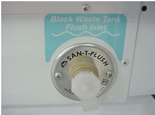
Water Tank Flush Inlet (typical)
