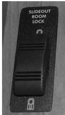
Slideout Room Locks - Typical Your model may be equipped with one or more types
