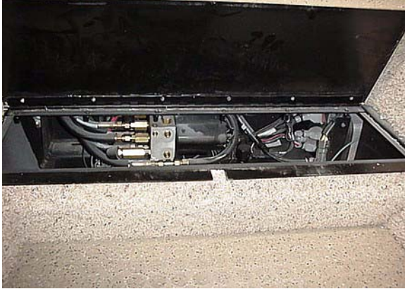
Hydraulic Pump Beneath Entry Step
