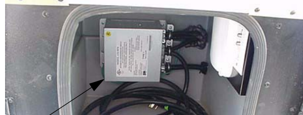
Automatic Power Transfer box in electrical utility compartment ( typical installation—appearance may differ on your model )
