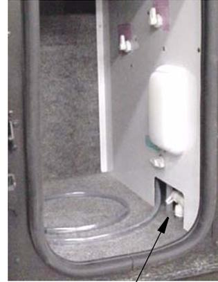
Water Line Drain Valve
