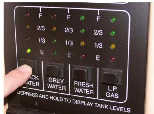
The approximate fluid levels are measured by sets of electronic sensors (detector cells) on the sides of the tanks. There is generally more fluid in a tank than indicated on the monitor panel.
