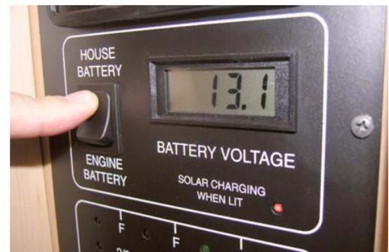
The LCD display will show the current battery voltage to the nearest tenth of a volt.
