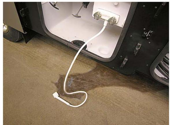
Using Exterior Shower to drain waterline
