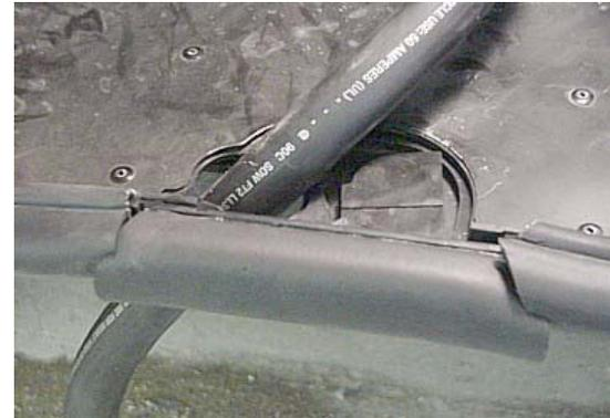
3. Route the cord through the notch and flip the hatch back up into place and close the compartment door.
