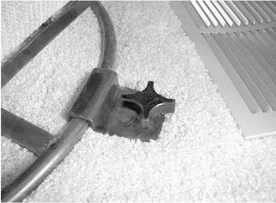
You can unscrew the knob and remove the clamp to position the chair where you desire in the living area of the coach.
