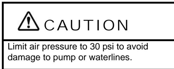
*NOTE: DO NOT burst air into the system. This can damage the water pump. It is better to let air in slowly.*
