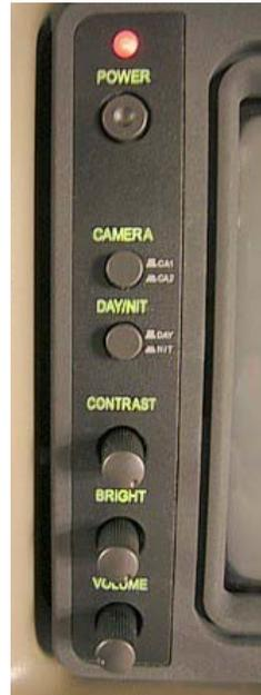
**Power** - Turn ON to activate monitor for rear viewing while driving or parked. Key must be on. In OFF position the monitor is 'asleep' and will 'wake up' when the transmission is shifted into Reverse.
