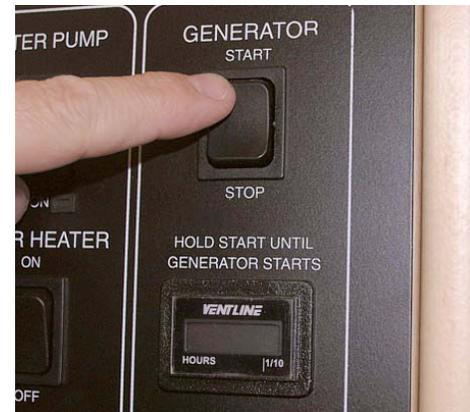
Generator Switch and Hourmeter on monitor panel
