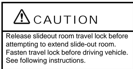
Some slideout rooms are equipped with electric powered travel locks to restrict movement of the slideout room while the vehicle is in motion.
