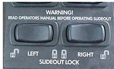
*Note: Be sure locks are fully released. The room will not extend or retract if the locks are protruding more than 1/4", and you will hear the slideout hydraulic pump running in idle/bypass mode when attempting to extend or retract room.*
