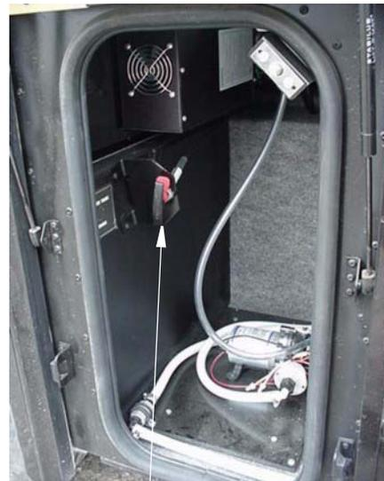
Water Tank Drain Valve- Model 38J
