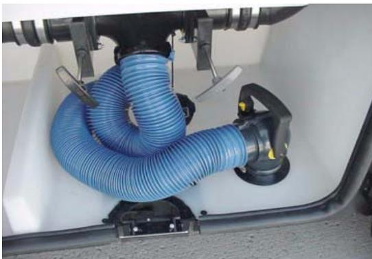
*NOTE: If the hose will not collapse while storing, open the hose end valve (handle) to release air trapped inside the hose.*
