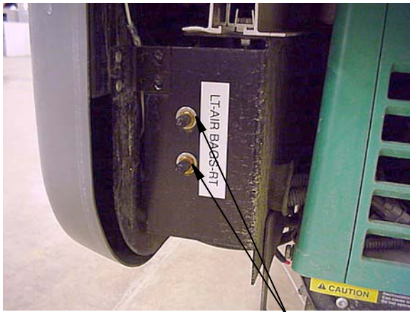
Rear Air Spring Fill Valves located on panel in generator compartment
