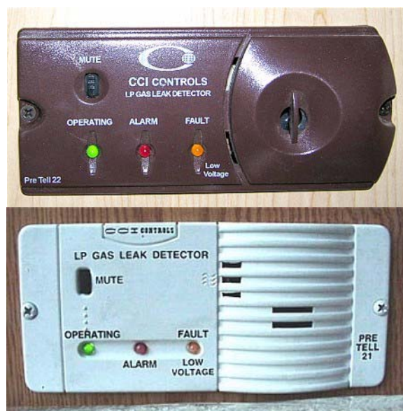
Propane Gas Leak Detectors (typical)
