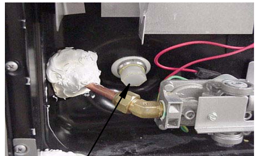
Water Heater Drain Plug (Remove with socket)
