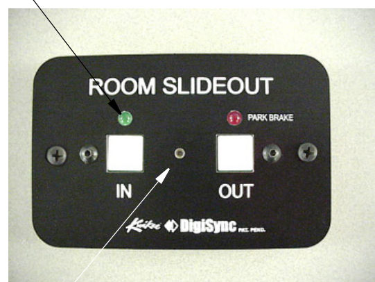
Reset Button -push with toothpick or plastic rod
