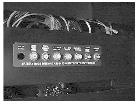
Chassis and House 12V Circuit Breakers behind cover panel in cargo compartment
