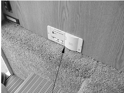
LP Gas Leak Detector
