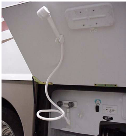
Exterior Shower/Wash Station (Typical)
