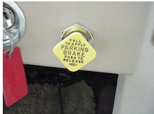
The pull-button knob can be used to apply the park brake when the coach is in any other gear than Park. Pull to apply. Push in to release.
