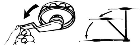
Turn elevating crank (counterclockwise) in "DOWN" direction until resistance is noted. Antenna is now locked in travel position. Turn amplifier power switch "OFF".
