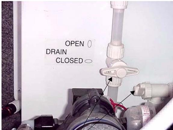
Water Line Drain Valves
