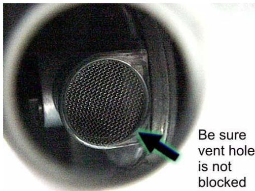
Regulator freeze-ups are caused by the presence of moisture in fuel. This moisture will pass through the cylinder valve and into the regulator where it can freeze. Fuel producers, tank and bottle manufacturers and LP gas dealers take every precaution to reduce moisture, but sometimes only a fraction of an ounce entering the tank can cause problems. To help avoid the possibility of freeze-up, always keep tank control valve closed when not in use, even when tank is
