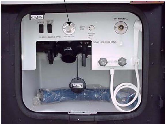
4. Turn the water on to begin flushing; allow water to run for about three minutes.
