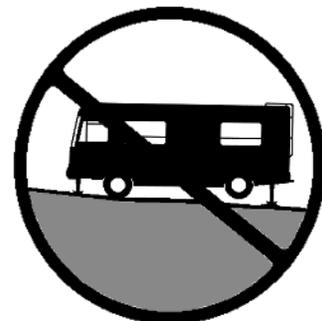
*NOTE: When parking at an uneven site, always park the front of the motor home to the downhill side. This allows you to level by raising the front end rather than the rear. Since only the rear wheels are locked while in PARK, raising either one or both of the rear wheels off the ground could allow the vehicle to roll off the jacks.*
