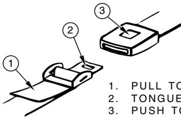
**Adjustment:** To lengthen belt, turn tongue at a right angle to belt and pull to desired length. To shorten, pull loose end of belt.
