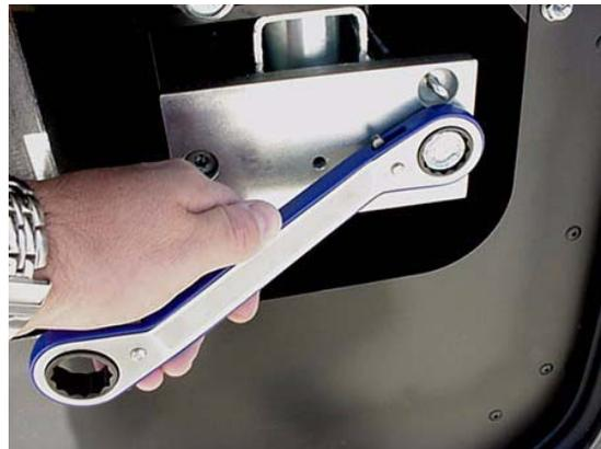
Crank the wrench(es) clockwise slowly, until the room is fully retracted. Allow about 10 minutes to crank room in fully.
