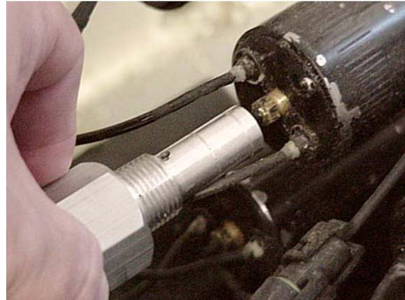
**IMPORTANT:** Prior to removing the breather cap, either to check the oil level or to use the 1/4" nut driver, clean any debris from the top of the reservoir before returning the breather cap to the reservoir. Remove any paint chips or other debris from the dipstick including debris inside the 1/4" nut driver.
