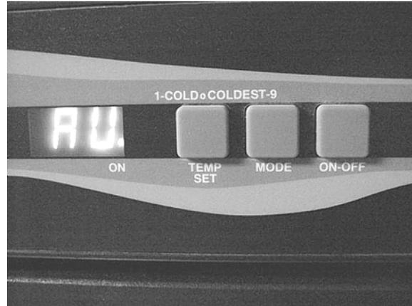
The ON/OFF button turns the refrigerator on or off. If the button is pressed, it will turn the refrigerator on and set the mode to auto. When the refrigerator is on, pressing this button for 2 seconds will turn the refrigerator off.
