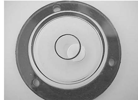
If over 1/2 of the bubble is inside the circle in any direction, the coach is level enough for continuous operation of the refrigerator while parked.
