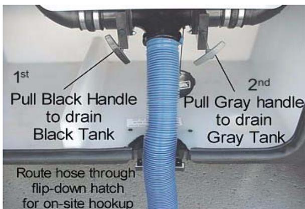
When using a sewer hook-up, keep the dump valves closed until a tank becomes full or when preparing to leave the site. This keeps the solids in suspension, allowing them to be carried out with the liquids when the dump valve is opened. If the valve is left open, the liquids will drain off,
