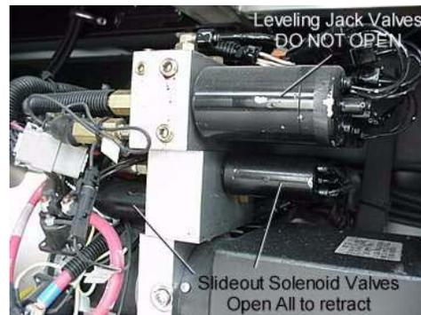
Leveling/Slideout System Hydraulic Pump
