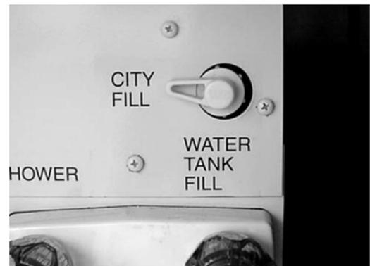
*NOTE: Because city water pressure varies from location to location, we recommend using an in-line water pressure regulator to prevent damage to any components, connections and seals in your fresh water system.*
