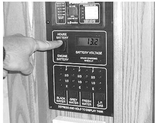
The LCD display will show the current battery voltage to the nearest tenth of a volt.
