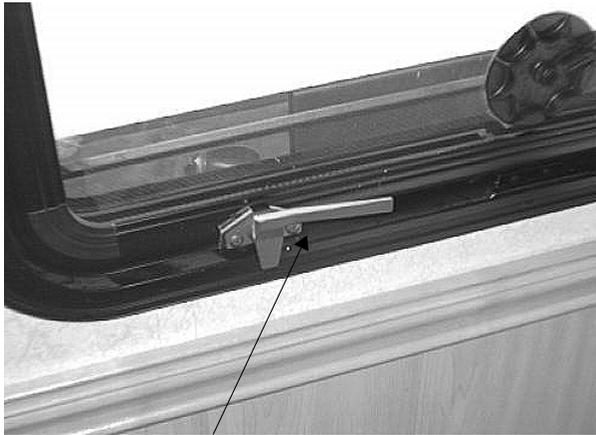
Lift latch handles upward to open.
