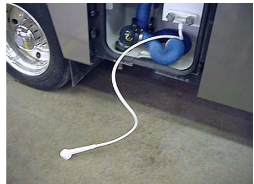
Models 32T & 39K: Place the exterior shower head on the ground and open the shower faucets to drain the water lines on these models.
