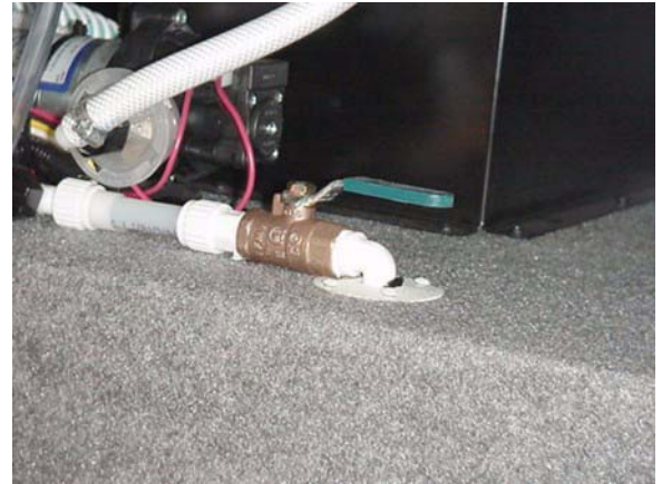
Water Line Drain Valve in RH Exterior Water Pump Compartment All models have this drain plus one of the following depending on models.
