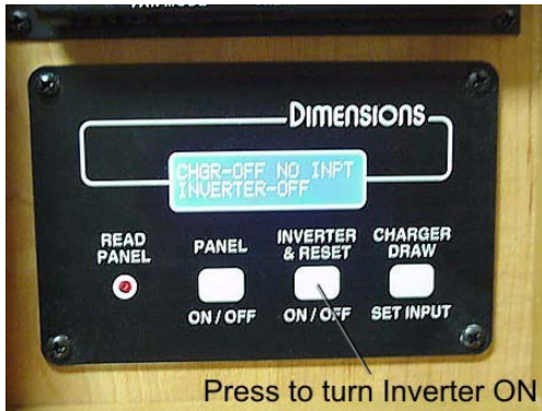
Inverter Charger Control Panel
