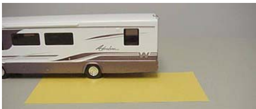
Weighing Left Rear 'Corner'
