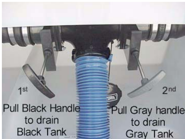
Holding Tank Valves (Typical)
