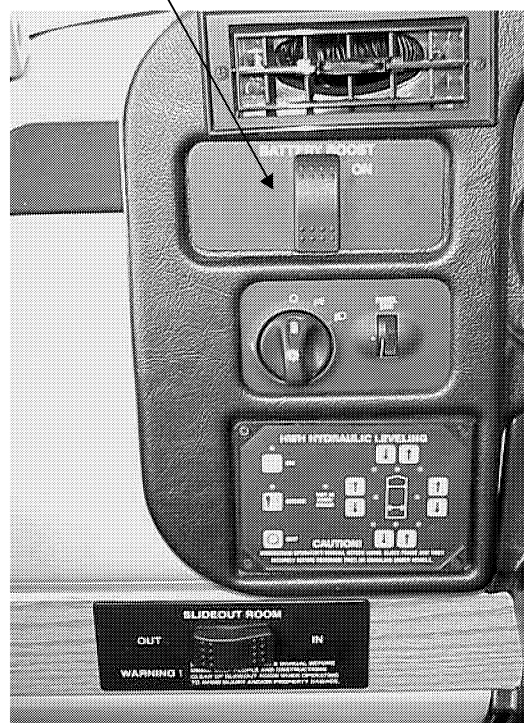
Battery Boost Switch
