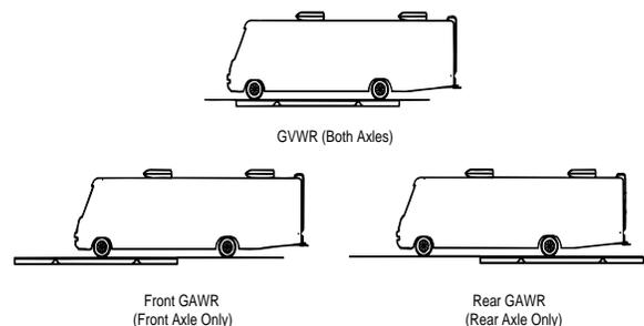
To determine the weight on either front or rear axle, drive that axle only onto the scale. Neither axle weight should exceed the corresponding maximum axle weight rating specified on the certification label.
