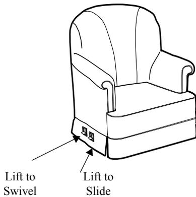
Swivel: Pull up on the swivel lever located on the side of the seat. The seat will lock into place whenever it reaches the center aisle facing position.
