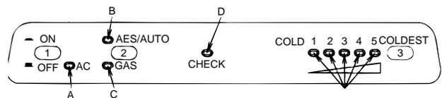
When operating in the GAS mode in the AES/AUTO mode indicator lamp (B) will be off and the Gas mode indicator lamp (C) will be illuminated. This mode provides LP gas operation only. The control system will activate the ignition system and will attempt to light the burner for a period of approximately 45 seconds. If unsuccessful, the CHECK indicator lamp (D) will illuminate and the GAS mode indicator lamp (C) will turn off.
