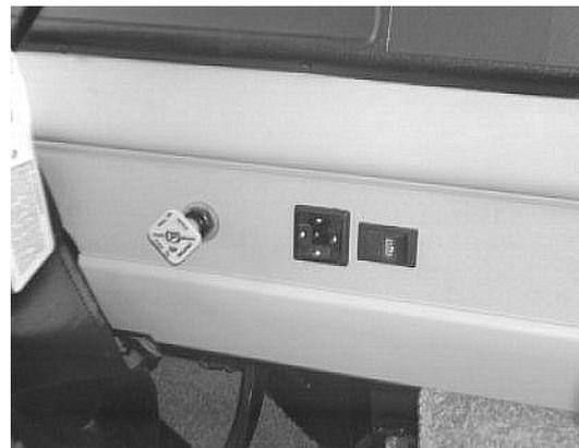
Use the parking brakes whenever the vehicle is parked. Never try to drive the vehicle with the park brake applied. This can cause excessive wear on the brakes and may damage the transmission.
