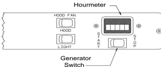
*NOTE: While the generator is running it is normal for the hourmeter to make a periodic "ticking" sound.*
