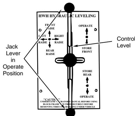
4. Extend the hydraulic jacks by pushing the center Control Lever to Front Raise, then Rear Raise. A corresponding, red warning light will glow as each jack is in position.
