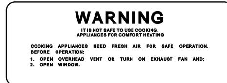
Unlike large homes, the oxygen supply inside a recreational vehicle is limited due to its size. To avoid danger of asphyxiation, provide proper ventilation when using the gas rangetop or gas oven. It is especially important not to use the gas oven and range top for comfort heating. Danger of asphyxiation is greater when these appliances are used for long periods of time.
