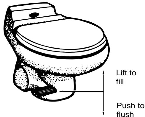
2. To flush the toilet, push the lever all the way down until sewage leaves the toilet and bowl is rinsed clean.
