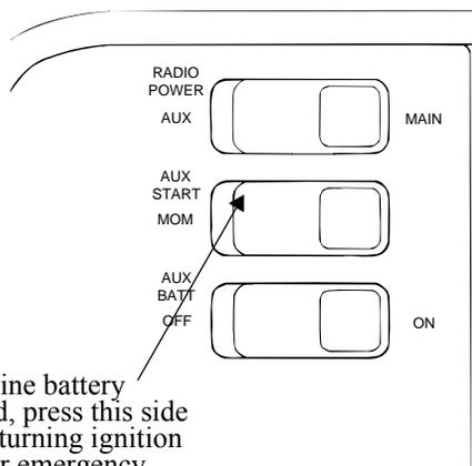
If engine battery is dead, press this side while turning ignition key for emergency starting power.
