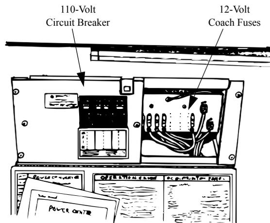
The fuse panel accepts only blade type plug-in fuses. Always replace fuses with those of the same amperage rating.
