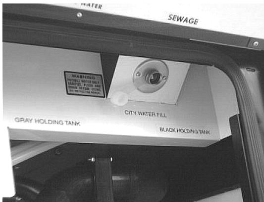
When connected to an outside source of water, the water bypasses the demand pump and storage tank and supplies pressure directly to individual faucets and toilet. A check valve built into the pump prevents water from entering the pump and filling the storage tank.
