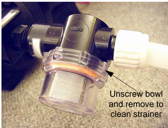
Water Pump Strainer -Typical View
