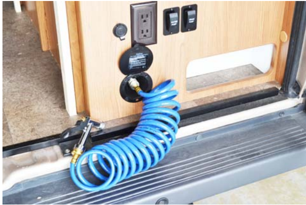
Exterior Shower/Wash Station (Typical)
