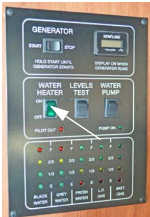
Electric Water Heater Switch (Located on Systems Monitor Panel)
