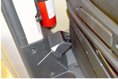
Second Power Awning Switch (if equipped) (Located near right side of passenger seat) -Typical View
