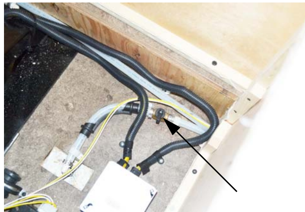
Water Tank Drain Valve (Located beneath forward facing dinette seat cushion) -Typical installation shown
