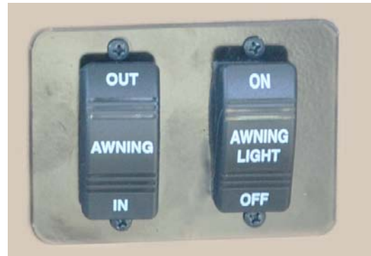
Power Awning Switch and Awning Light Switch (if equipped) (Located at front of galley or shower wall) -Typical View
