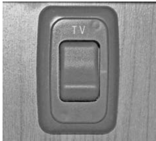
12-Volt TV Master Power Switch (Located in overhead cabinet behind the Swing Out TV) -Typical View
