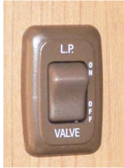
LP Tank Valve Switch
