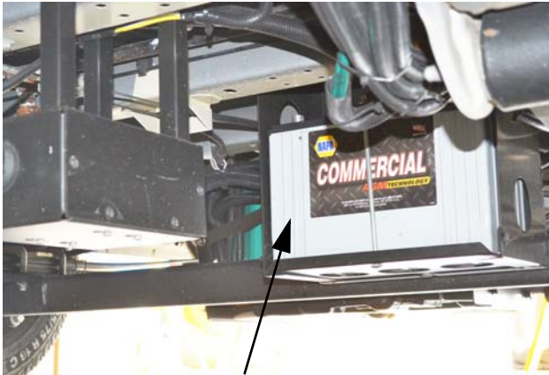
House Battery Access (Located behind rear tires) - Remove bolts from battery retainer to remove house battery
