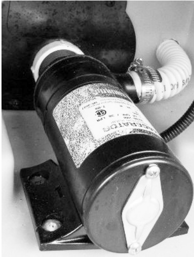
Waste Pump (Located beneath coach) -Typical View
