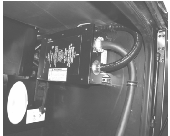
Automatic Power Transfer Box (Located inside or behind utility compartment) -Typical installation shown
