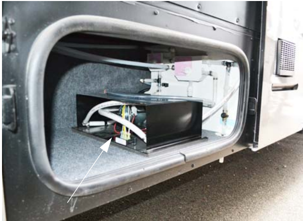
Water Pump (Located in compartment behind entrance door) * Models 32H and 35P shown
