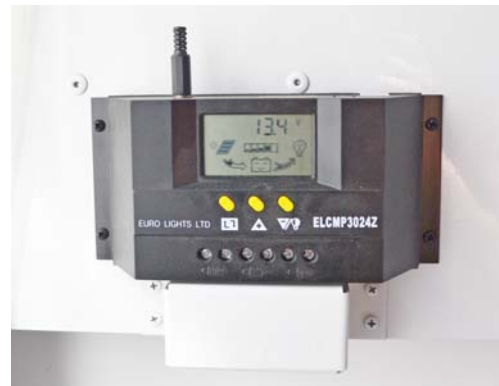
Solar Charge Controller (Located in utility compartment)
