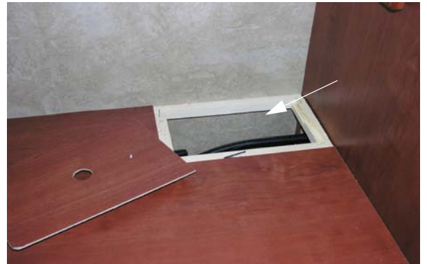
Water Supply Faucets (Located below access panel in wardrobe) * Model 38Q shown
