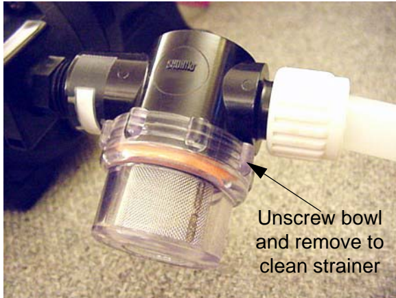
Water Pump Strainer -Typical View
