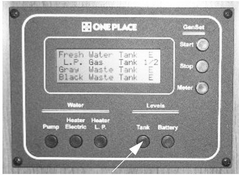
Tank Levels Switch
