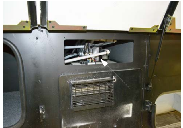
Water Pump (Located on passenger side above water heater. Remove water heater door to access.) * Model 38Q shown
