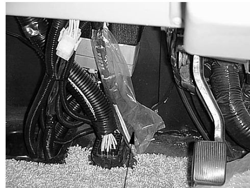
CB Power Wires (in plastic sheath) Typical view - your coach may differ slightly
