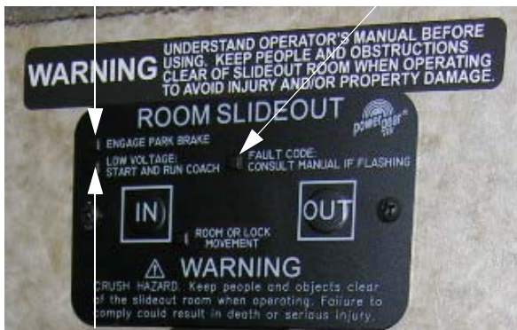
Low Voltage Indicator
