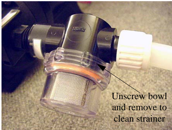
Water Pump Strainer -Typical View
