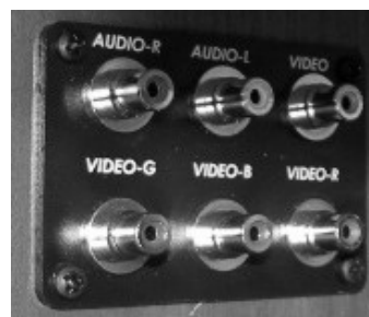
Audio Video Connection Plate -Typical View
