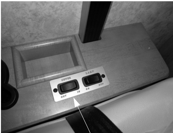
Step Cover Switch -Typical View
