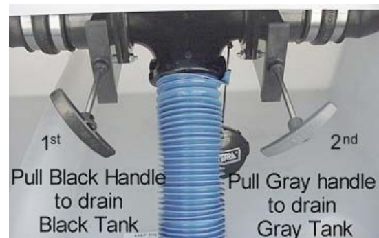
Holding Tank Dump Valves -Typical View
