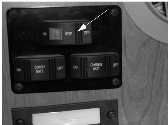
Entry Step Switch - Typical * Model D31E shown (Located near the entrance door)
