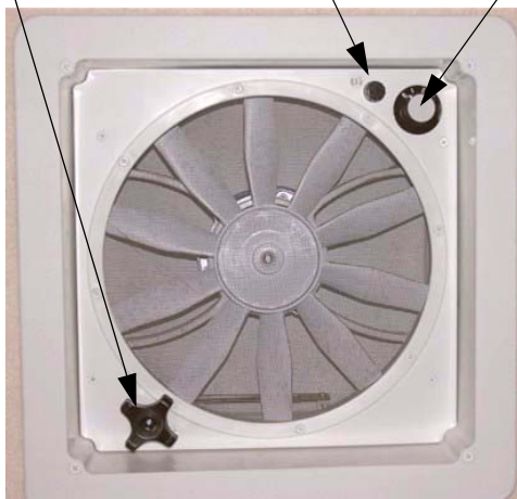
Power Roof Ventilator
