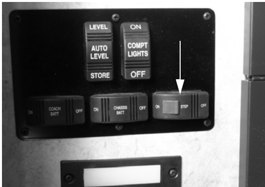
Entry Step Switch - Typical (Located near the entrance door)
