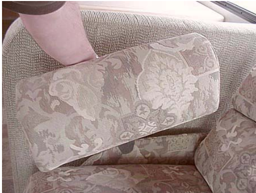
Remove armrest by pulling upward
