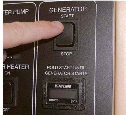
Generator Switch and Hourmeter on Monitor Panel
