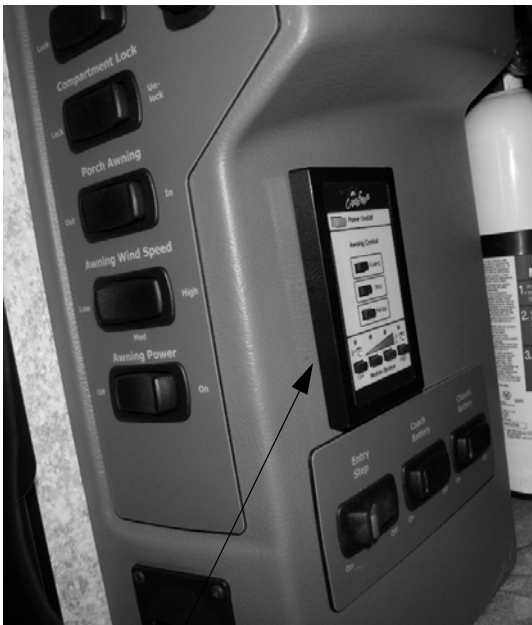
Awning Control Switch Panel - Typical View (Located near entrance door)
