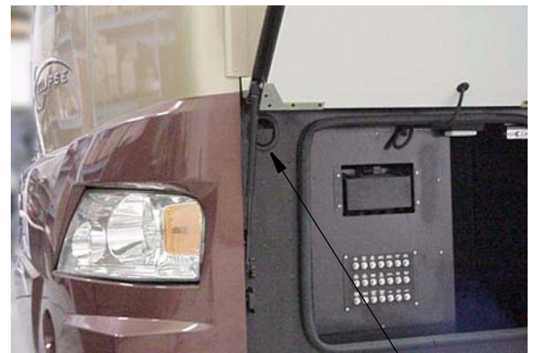
Hood Latch Location in 12-volt electrical compartment
