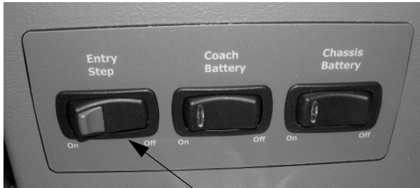
Entry Step Switch - Typical (Located near the entrance door)
