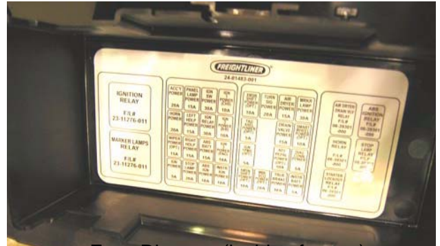
Fuse Diagram (inside of cover)
