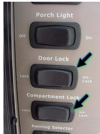
Power Door Locks on entry switch panel
