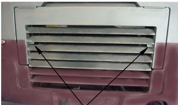
Lift latches and swing grille upward
