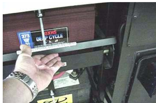
Lift Battery Tray Retainer Latches
