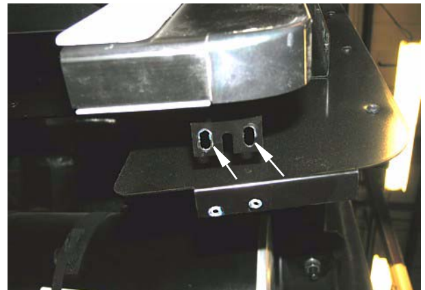
Remove 2 screws in lower rear edge of grill panel shown, then swing hinged panel upward.
