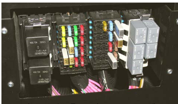
Automotive Fuses (cover removed)
